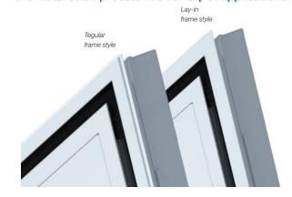
SHP Diffusers feature a 1 in. discharge slot with dual layer pattern controllers that can be field adjusted from the diffuser face.
